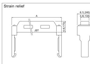
Cover housing For long locking lever header
